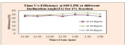
An experimental study has been carried out to investigate the efficiency of solar flat plate collector using  $BN/H_2O$  nanofluid. The volume concentration of  $BN/H_2O$  nanofluid has been varied from 1 % to 3 %. The performance of solar flat plate collector was evaluated at different inclination angle. The effete of mass flow rate on the performance of solar flat plate collector has also been investigated.
